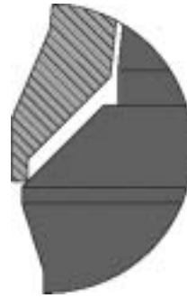
Coping following casting. The snap-on mechanism no longer works. The lip must be removed before the cast coping is placed on the analog.
